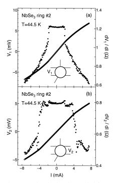
Fig. 1. Voltages  $V_1$  and  $V_2$  developed across the left (a) and right (b) arms of the ring-shaped crystal plotted as a function of the total current through the ring. Current derivative of  $V_1$  and  $V_2$  are also shown.
