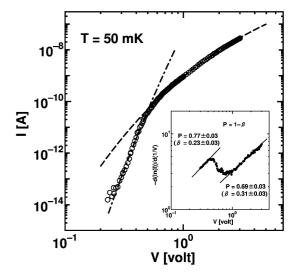
Fig. 3. The bias dependence of the nonlinear current observed at 50 mK. The dashed line is a scaling form  $I = I_0 \exp[-(V_0/V)^\beta]$  with  $\beta = 0.31$ ,  $I_0 = 1.23 \times 10^{-4} \, \text{A}$ ,  $V_0 = 2.84 \times 10^3 \, \text{V}$ . The dashed-and-dotted line is the same form with  $\beta_2 = 0.23$ ,  $I_0 = 1.27 \times 10^{11} \, \text{A}$ , and  $V_0 = 1.14 \times 10^7 \, \text{V}$ . The inset shows the plot of  $-\text{d}(\ln I)/\text{d}(1/V)$  vs V on a log-log scale.
