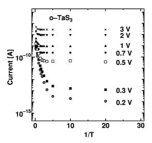
Fig. 2. The temperature dependence of the current I(T) measured at various electric fields.
