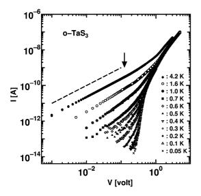
Fig. 1. I-V characteristics of o-TaS<sub>3</sub> in the temperature range of  $50\,\mathrm{mK}\text{-}6\,\mathrm{K}$ . The dashed line corresponds to ohmic behavior. The threshold field is indicated by the arrow.
