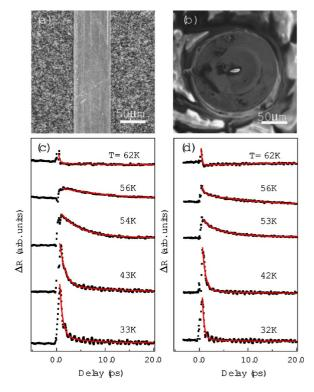
FIG. 1. (Color online). Electron micrographs of the topological samples: (a) Whisker and (b) ring. The corresponding transient reflectivity changes,  $\Delta R$ , at various temperatures below and above  $T_{c2}$  in (c) and (d). The solid lines indicate the results of least-squares fitting.
