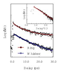
FIG. 3. (Color online) Semilogarithmic plots of the reflectivity changes for the whisker (T=56 K) and the ring (T=52 K), where the longest  $\tau_s$  was obtained in each crystal. The plots are shifted vertically for clarity. The inset shows another plot for the ring. The solid line indicates the slope of  $\exp(-t/\tau)^{0.3}$ , where  $\tau$  is 1.61.
