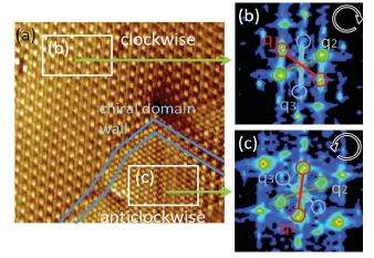
FIG. 2 (color). (a) 12 nm  $\times$  12 nm STM image and (b),(c) FT of two areas each enclosed with a square in sample *B*. Sample *B* was measured at  $V_s = -350$  mV and  $I_t = 0.4$  nA at T = 6.3 K. The blue line is the domain wall between the clockwise phase and the anticlockwise phase.
