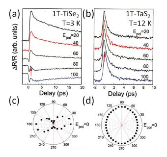
FIG. 3 (color online). Polarization dependence of transient reflectivity variation in 1T-TiSe<sub>2</sub> measured at 3 K (a) and 1T-TaS<sub>2</sub> measured at 12 K (b). The height of each peak is plotted in the (c) and (d) as function of polarization angle  $E_{\rm pol}$ . The pump pulse wavelength is 1160 nm and the power is 150  $\mu$ W. The probe pulse is 800 nm, 80  $\mu$ W.
