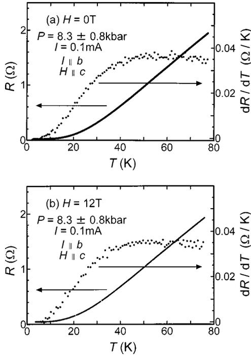
FIG. 3. Temperature dependence of the resistance  $R$  and its temperature derivative  $dR/dT$  at (a)  $H=0$  T and (b)  $H=12$  T at  $P=8.3 \pm 0.8$  kbar. The superconductivity appears at  $T_s=2.5$  K at  $H=0$  T.
