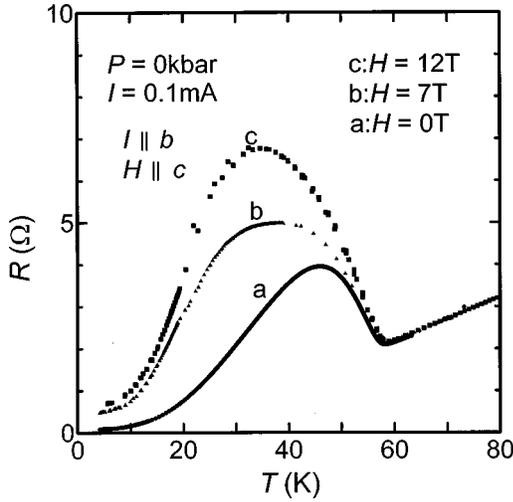
FIG. 1. Temperature dependence of the resistance in the range 2–80 K at ambient pressure at  $H=0, 7,$  and  $12$  T.
