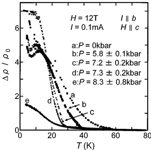
FIG. 4. Temperature dependence of the magnetoresistance  $\Delta\rho/\rho_0$  at various pressures in the magnetic field of 12 T.
