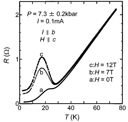
FIG. 2. Temperature dependence of the resistance in the range 2–80 K at  $P=7.3\pm 0.2$  kbar at  $H=0, 7,$  and  $12$  T.
