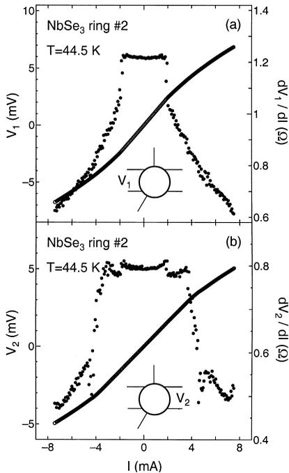
Fig. 1. Voltages  $V_1$  and  $V_2$  developed across the left (a) and right (b) arms of the ring-shaped crystal plotted as a function of the total current through the ring. Current derivative of  $V_1$  and  $V_2$  are also shown.
