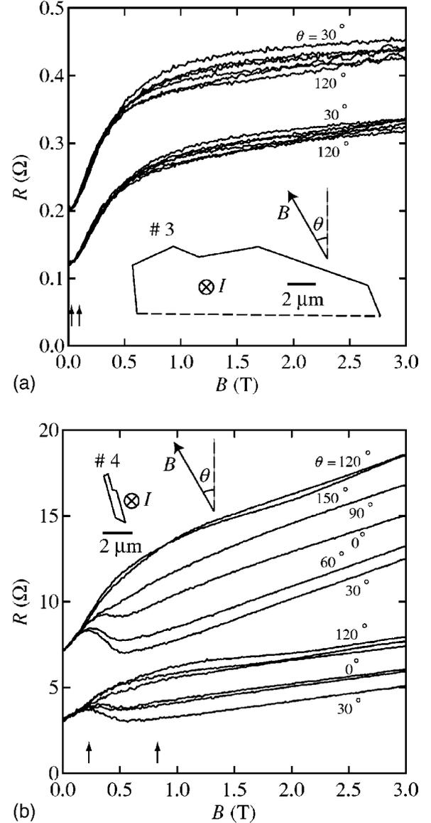
FIG. 2. The magnetoresistance of (a) thick (3) and (b) thin (4) crystals, measured at 0.28 K for the field orientations  $\theta=0^\circ$ ,  $30^\circ$ ,  $60^\circ$ ,  $90^\circ$ ,  $120^\circ$ , and  $150^\circ$ . The  $c$  axis corresponds to  $\theta=98^\circ$  for sample 3 and  $\theta=36^\circ$  for sample 4. The arrows indicate the magnetic fields  $B=0.55\hbar\sqrt{S_{a^*b^*}}/\pi/ed_{a^*}$  and  $2.0\hbar\sqrt{S_{a^*b^*}}/\pi/ed_{a^*}$ .
