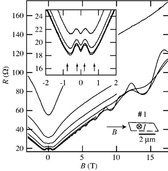
FIG. 1. The magnetoresistance of a NbSe<sub>3</sub> crystal with 0.49 μm thickness (sample 1) at several temperatures;  $T=16.00$  K, 12.00 K, 10.00 K, 8.00 K, 6.00 K, 4.00 K, and 0.28 K from the top curve to the bottom one. Inset: An enlargement of the low-magnetic-field region.  $T=8.00$  K, 6.00 K, 4.00 K, and 0.28 K from top to bottom. The arrows indicate the magnetic fields  $B=0.55\hbar\sqrt{S_{a^*b^*}}/\pi/ed_{a^*}$  and  $2.0\hbar\sqrt{S_{a^*b^*}}/\pi/ed_{a^*}$ .
