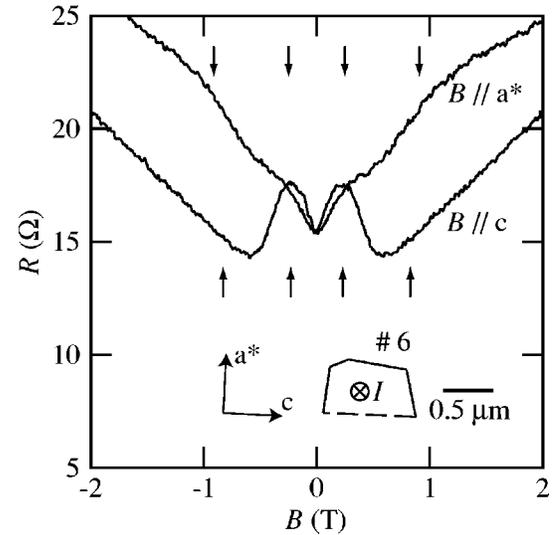
FIG. 4. The magnetoresistance of sample 6 at  $T=1.72$  K. This sample has the narrowest width along the  $c$  axis. The upward arrows indicate the magnetic fields  $B=0.55\hbar\sqrt{S_{a^*b}/\pi}/ed_{a^*}$  and  $2.0\hbar\sqrt{S_{a^*b}/\pi}/ed_{a^*}$ , while the downward arrows indicate  $B=0.55\hbar\sqrt{S_{b^*c}/\pi}/ed_c$  and  $2.0\hbar\sqrt{S_{b^*c}/\pi}/ed_c$ .
