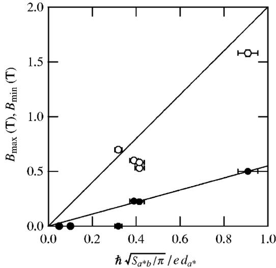
FIG. 3. The magnetic fields  $B_{\max}$  and  $B_{\min}$ , where the magnetoresistance curves show a maximum and a minimum, plotted as a function of  $\hbar\sqrt{S_{a^*b}/\pi}/ed_{a^*}$ . The closed and open circles show  $B_{\max}$  and  $B_{\min}$ , respectively. The solid lines have slopes of 0.55 and 2.0.
