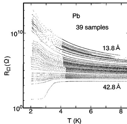
FIG. 1. Resistance of the samples vs temperature. The film is grown sequentially *in situ* by evaporation of Pb. The film changes to superconductor from insulator as film thickness increases. Film thickness changes from 13.8 to 42.8 Å. The superconducting transition takes place at 3.5 K in the thickest film.
