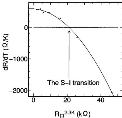
FIG. 3. Temperature coefficient of resistance (TCR) vs sheet resistance at 2.3 K. The sheet resistance is a parameter of the degree of disorder in the films. A positive TCR indicates that a film becomes a superconductor ( $T \rightarrow 0$ ) and a negative TCR indicates that a film becomes an insulator ( $T \rightarrow 0$ ). The SI transition takes place at the point where TCR is zero.
