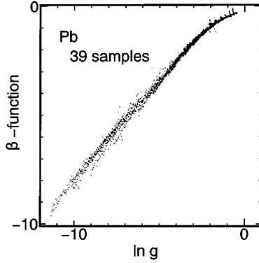
FIG. 4. The  $\beta$  function vs dimensionless conductance for all films above 4 K. This figure shows that the conductance of all films studied fit a single universal curve. This confirms that all films are in the fermion region above 4 K. Below 4 K, data cannot be fitted to a single universal curve.
