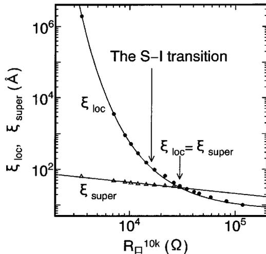
FIG. 5. The superconducting coherence length ( $\xi_{super}$ ) and the electrical localized length ( $\xi_{loc}$ ) vs the sheet resistance at 10 K. The sheet resistance at 10 K is a parameter of the degree of disorder in the films. The SI transition takes place at a point where  $\xi_{loc} \approx 2\xi_{super}$ , and the criterion that the SI transition takes place at the point where  $\xi_{loc} = \xi_{super}$  is not observed.
