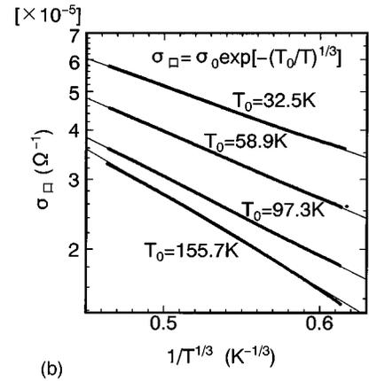
FIG. 6. (a) Conductance vs temperature for superconducting films. The conductance shows logarithmic temperature dependence. This indicates that the films are weak-localized regimes. Observed coefficient of  $\ln T$  is  $2.59 \times 10^5$  and the value of  $p$  is 2.1. (b) Conductance vs temperature for insulator films near the SI transition. The conductance shows VHR transport  $1/\sigma_{\alpha} \propto \exp[-(T_0/T)^{1/3}]$ .  $T_0$  is the general activation energy.
