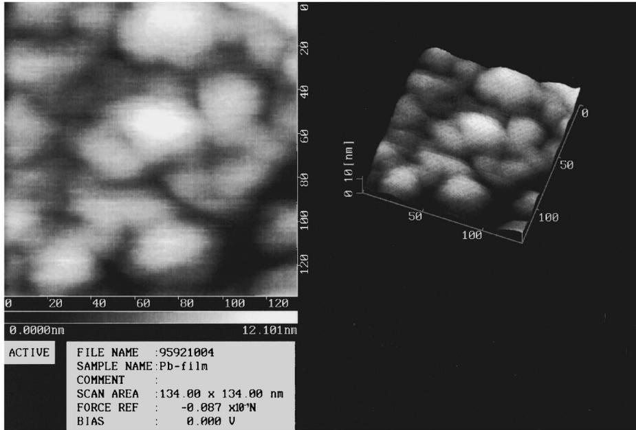
FIG. 2. AFM topography of the thickest (42.8 Å) film. This value represents the average Pb grain height. The thicknesses of other films is calculated from the evaporation time.
