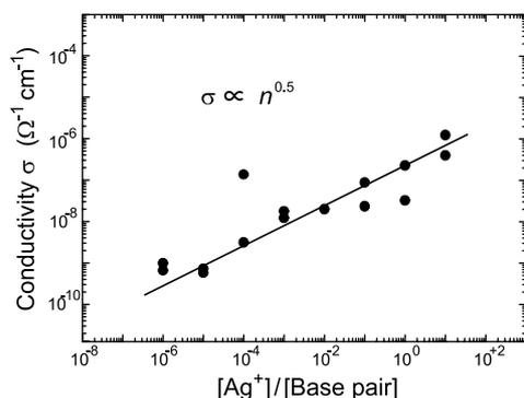
Fig. 4. Dependence of electrical conductivity of Ag-doped DNA on  $[Ag^+]$ . The solid line represents  $\sigma \propto n^{0.5}$ . The electrical conductivity of non-doped DNA is  $(8.24 \pm 2.06) \times 10^{-10} \Omega^{-1} \text{cm}^{-1}$ .
