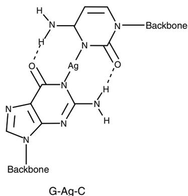
Fig. 1. Schematic representation of the binding site of  $\text{Ag}^+$  in Ag-doped DNA [15].  $\text{Ag}^+$  forms two covalent bonds with two nitrogen atoms in G-C pairs and then takes electronic structure of  $4d^9 5s^1 5p^1$ .
