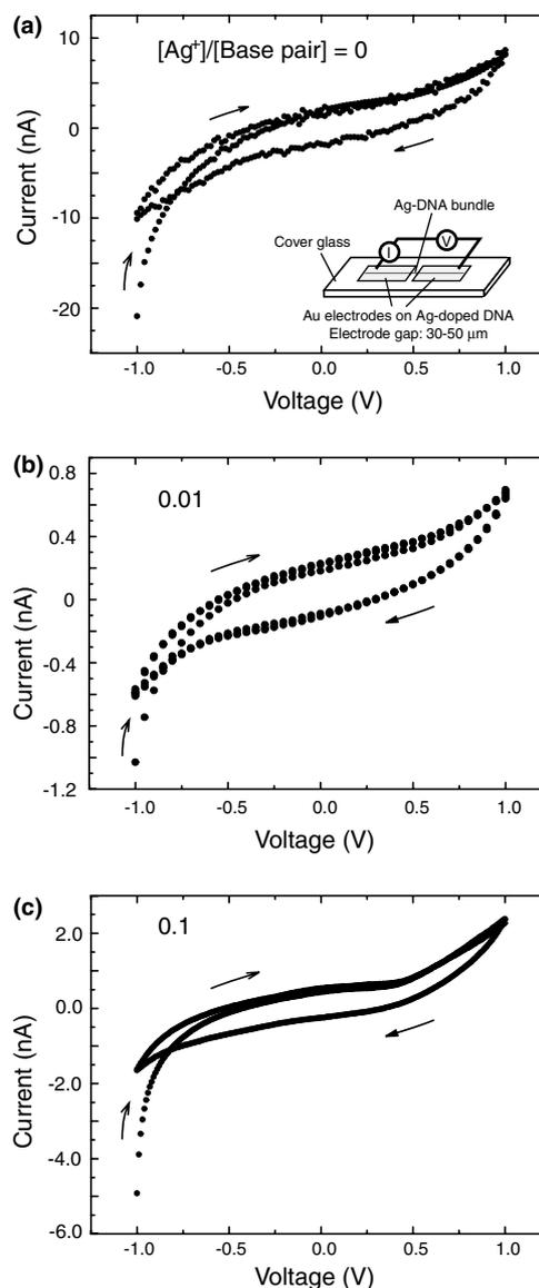
Fig. 3. Typical  $I$ – $V$  curves observed in Ag-doped DNA at  $[Ag^+]/[Base\ pair] = 0$  (non-doped DNA) (a); 0.01 (b); 0.1 (c) within  $\pm 1\ V$ . Arrows indicate the direction of bias voltage tuning and the inset shows a schematic representation of a sample set.
