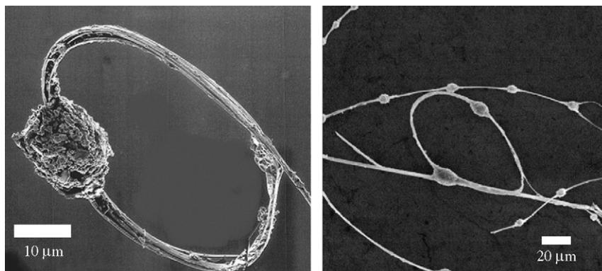
Fig. 3. SEM images of ring-shaped crystals of TaSe<sub>3</sub> with Se condensates (droplets), which seem the starting form of the successive spooling mechanism in Fig. 2D. They are the strong evidence for the formation mechanism of linked rings of crystals proposed in this paper.
