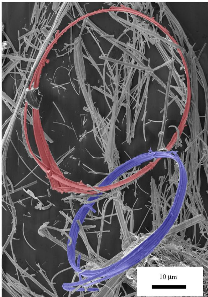
Fig. 1. Scanning electron microscope (SEM) image of linked rings of crystal formed of a compound of tantalum and selenium ( $\text{TaSe}_3$ ). The blue and red rings have respective diameters of 46 and 54  $\mu\text{m}$ . The two rings are linked with each other exactly once.
