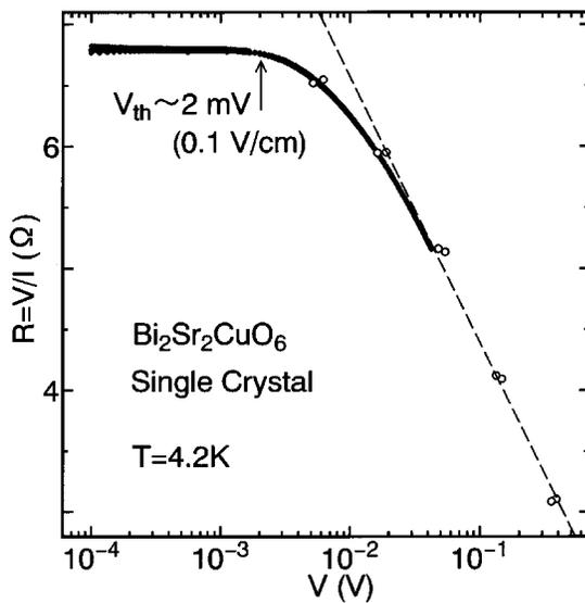
FIG. 2.  $I$ - $V$  characteristics of the sample at 4.2 K, plotting  $R(=V/I)$ . Dots and open circles represent data obtained by dc and pulse measurement, respectively. Both values agree around  $10^{-2}$  V. Resistance  $R$  remains constant below the threshold electric field, at which  $R$  begins increasing by  $\ln T$ .
