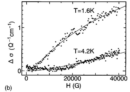
FIG. 3. (a) The transverse and longitudinal magnetoresistances of sample. Note that the sign of magnetoresistances is negative for both directions. (b) The component of orbit motion contributing to magnetoconductivity,  $\Delta\sigma = -(\Delta\rho_T - \Delta\rho_L)/\rho_0^2$ . Solid lines show the fit with theory.
