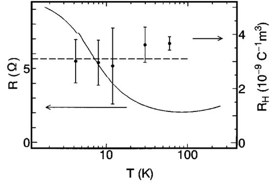
FIG. 4. Temperature dependence of Hall coefficients (solid circles) and resistance (solid line) of the sample. The Hall coefficients is almost independent of temperature (see text).
