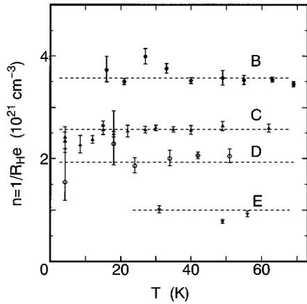
FIG. 3. Carrier concentration of samples B, C, D, and E, determined as  $n = 1/R_H$ , where  $R_H$  is the Hall coefficient. The carrier concentration becomes smaller when much Sr is substituted by Bi. It is shown that the Hall coefficient of each sample is independent of temperature.
