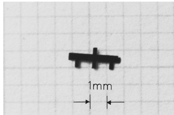
FIG. 1. A Hall-bar shaped  $\text{Bi}_{2+x}\text{Sr}_{2-x}\text{CuO}_y$  single crystal. The sample was cut by repeating step-by-step laser drilling. Sample size was 2.7 mm in length and 0.5 mm in width.
