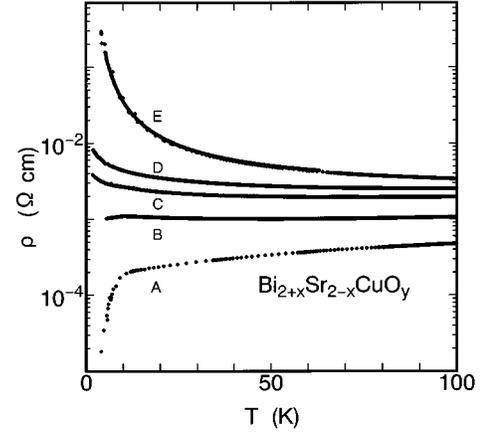
FIG. 2. Resistivities of the samples with different Bi/Sr ratio. The sheet resistance of  $1.0 \text{ k}\Omega$  corresponds to the resistivity  $1.2 \times 10^{-4} \Omega \text{ cm}$ . The residual resistivity becomes higher when much Sr is substituted by Bi. Sample B exhibits the weak localization, whereas C, D, and E show the variable range hopping conduction.
