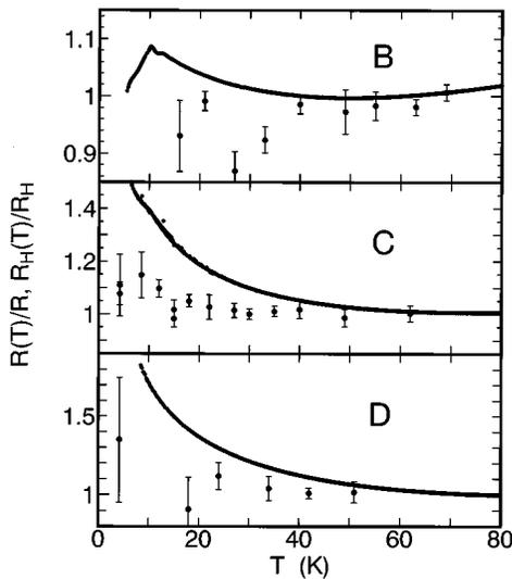
FIG. 4. Normalized resistivity  $\delta R(T)/R$  (solid lines) and Hall coefficient  $\delta R_H(T)/R_H$  (solid circles with error bars) of samples B, C, and D. If the Coulomb interaction plays a major role in resistivity upturn, the Hall coefficient should depend on the resistivity:  $\delta R_H(T)/R_H = 2\delta R(T)/R$ . The data shown here demonstrate no such dependency.
