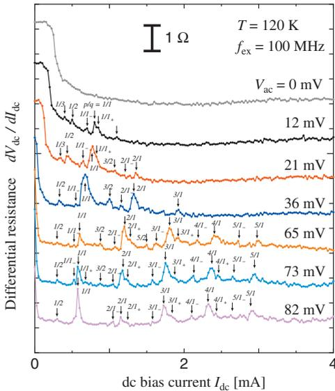
FIG. 2. (Color) dc bias current dependence of differential resistance  $dV_{dc}/dI_{dc}$  with applied various ac voltages of  $f_{ex}=100$  MHz at  $T=120$  K. The ac voltages  $V_{ac}$  are 0, 12, 21, 36, 65, 73, and 82 mV from top to bottom. Harmonic and subharmonic Shapiro steps are indicated by arrows and index  $p/q$ , where  $p$  and  $q$  are integers. Moreover, there are small beat peaks ( $p/q_-$  and  $p/q_+$ ) on both sides of the main Shapiro peaks.
