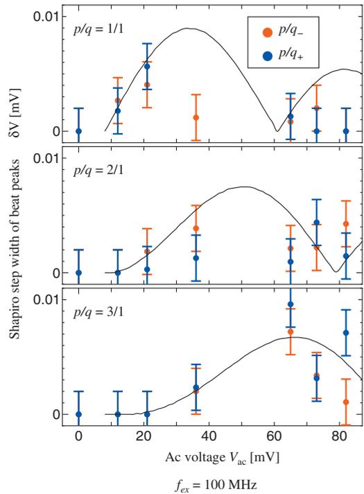
FIG. 4. (Color) ac voltage amplitude dependence of Shapiro step width  $\delta V$  of negative and positive beat peaks of (a)  $p/q=1/1$ , (b)  $2/1$ , and (c)  $3/1$ . The calculation curves of amplitudes of Bessel functions  $|J_1(x)|$ ,  $|J_2(x)|$ , and  $|J_3(x)|$  are the rescaled ones in Fig. 3.
