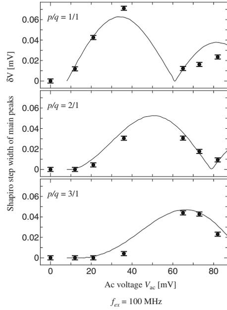
FIG. 3. ac voltage amplitude dependence of Shapiro step width  $\delta V$  of main peaks of (a)  $p/q=1/1$ , (b)  $2/1$ , and (c)  $3/1$ . The step width is estimated as the product of peak height and half width of half maximum of each peak of Fig. 2. Solid lines are calculation results of amplitudes of Bessel functions  $|J_1(x)|$ ,  $|J_2(x)|$ , and  $|J_3(x)|$ , respectively.
