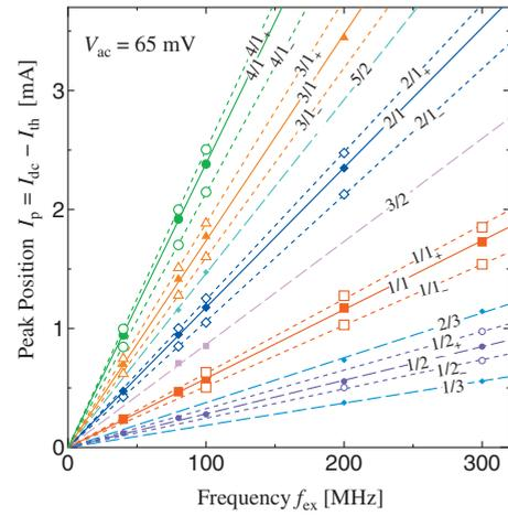
FIG. 6. (Color) Frequency dependence of peak position  $I_p=I_{dc}-I_{th}$  of each step. The peak positions of the harmonic, subharmonic, and beat peaks are proportional to frequency. The slopes of each line are shown as a function of the index  $p/q$  in Fig. 7.
