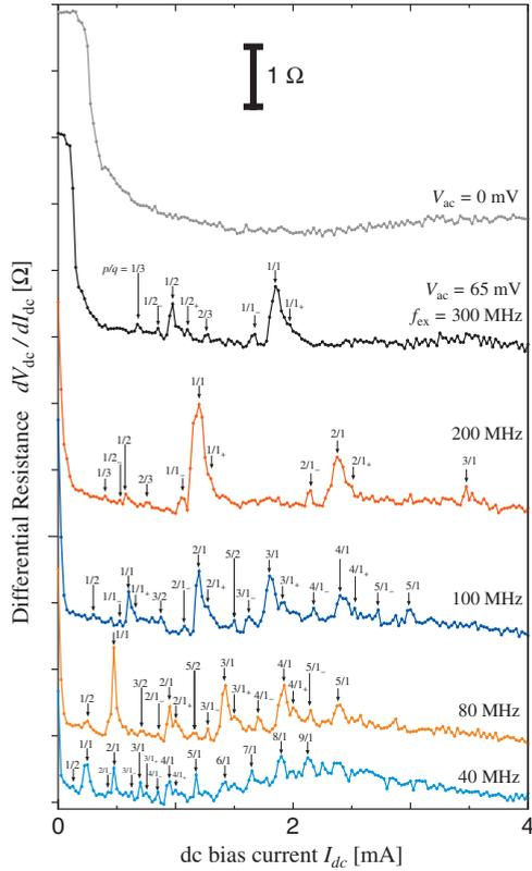
FIG. 5. (Color) Differential resistance  $dV_{dc}/dI_{dc}$  versus dc current  $I_{dc}$  at  $T=120$  K without ac voltage and with ac voltage of amplitude  $V_{ac}=65$  mV and frequency  $f_{ex}=40, 80, 100, 200,$  and  $300$  MHz, respectively.
