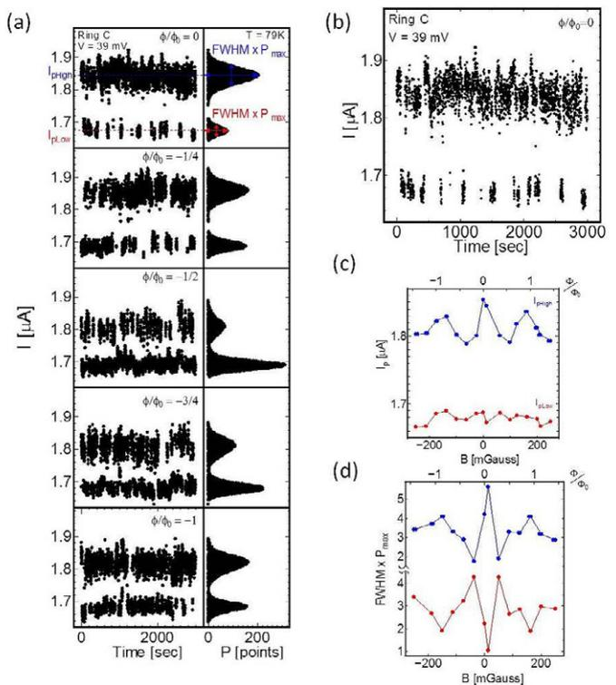
Fig. 4: (Colour on-line) (a) Time dependence of the electric current for applying constant voltages for 3000 seconds at 79 K. (b) Top panel of (a) zoomed in. (c) Peak currents of the two states as a function of the magnetic field. (d) The product of the full width at half-maximum (FWHM) and the peak height  $P_{max}$ , which correspond to the areas of the states.
