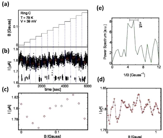
Fig. 3: (Colour on-line) Measurements and analysis technique. Time dependence of magnetic field (a) and the electric current (b). (c) Relation between the current and the magnetic field. (d) Current data applied with high magnetic field. (e) DFT performed on the time-averaged data  $I(B_i)$  to extract periodic components which depend only on the magnetic field.
