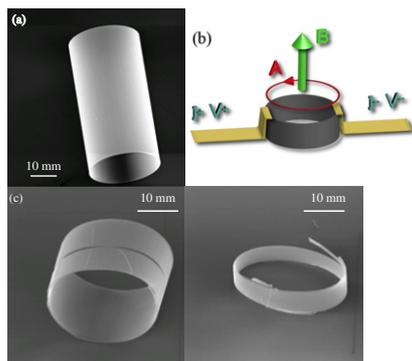
Fig. 1: (Colour on-line) (a) Scanning electron microscope (SEM) image of a TaS<sub>3</sub> tube-shaped crystal. (b) Contact configuration for transport measurement. Two gold electrodes (100 nm thick, 5 μm wide) were evaporated. (c) SEM image of a TaS<sub>3</sub> tube/ring crystal before cutting, (left) after cutting (right).
